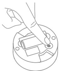
4. The resetting process is complete when the LED starts to flash.
