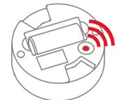
7. When the LED stops flashing, the Heat Alarm has successfully joined the ZigBoat™ network.
