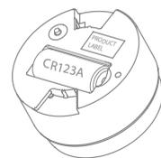
2. To find the serial number detach the sensor mount base.
